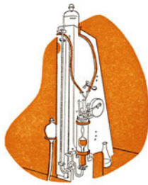
The Van Slyke apparatus is used in enzyme studies of cancer. For example, the enzymes of a tumor extract are allowed to act on peptides and the rate at which amino acids are formed is measured by this instrument.
