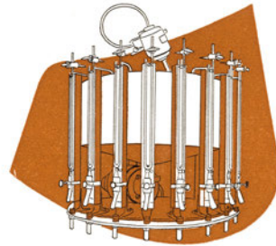
The Warburg apparatus is used in enzyme studies of cancer. The manometer measures the enzymatic activity in terms of gas exchange in a closed vessel submerged in the circular tank. Water in the tank is kept at body temperature to simulate natural conditions.
